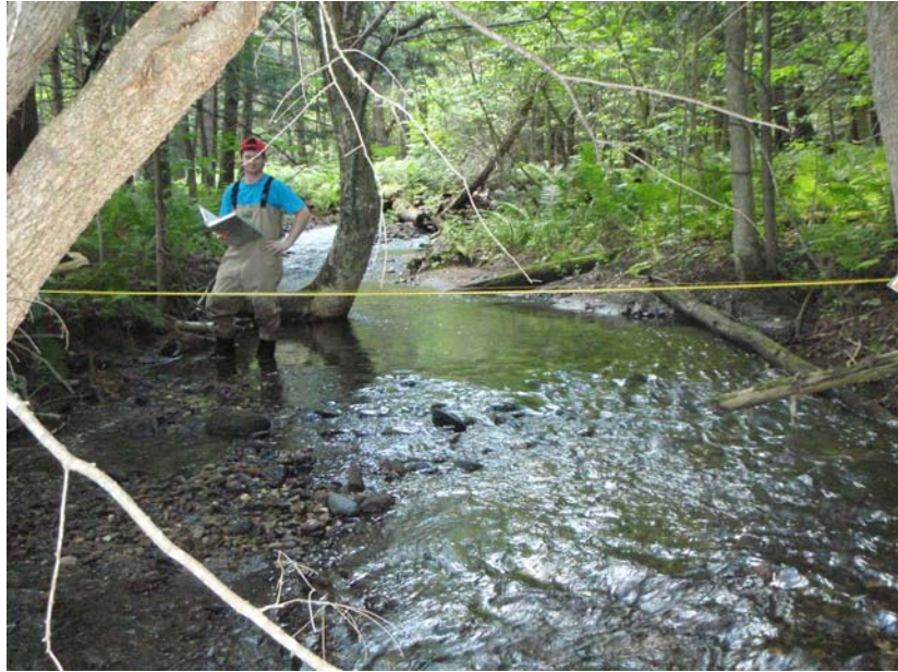
Figure 4.55 Cross-section looking upstream; C-type morphology and riffle-pool bedform
