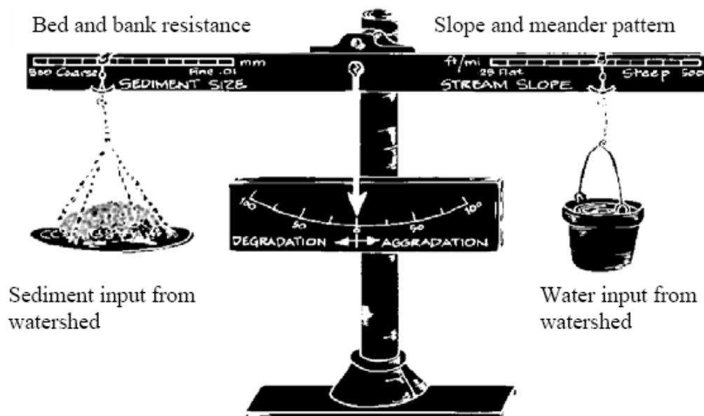
**Figure 13.** The channel balance indicates how changes in watershed inputs influence channel adjustment processes (Lane 1955).
