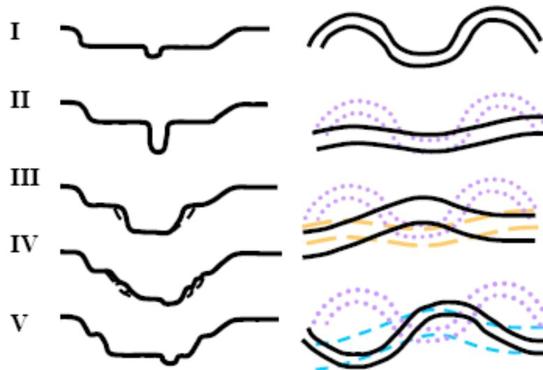
**Figure 28. Channel evolution process showing channel downcutting or incision in Stage II (cross section), widening through Stages III and IV, and floodplain reestablishment in Stage V. Stages I and V represent equilibrium conditions. Plan view shows straightening and meander redevelopment that accompany cross-section changes, a primarily flood-driven process often taking place over decades (VT-RMP\_ApxC 2007).**
