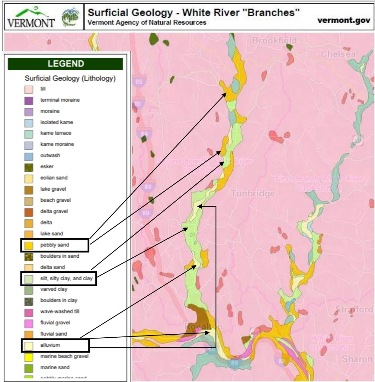
Figure 5. Surficial Geology (Lithology) of the White River “Branches”, highlighting preponderance of glaciolacustrine soils (especially ‘silt, silty clay, clay’) and other fine-grained soils along significant portions of the Second Branch.
